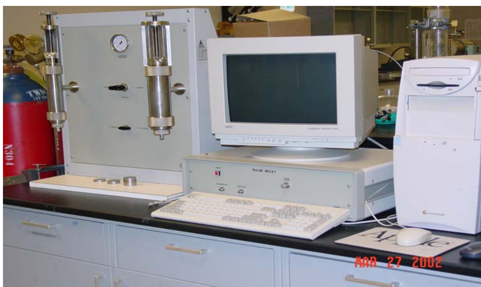
Figure 6 Pulse-decay Permeameter (Courtesy of CoreLab)
