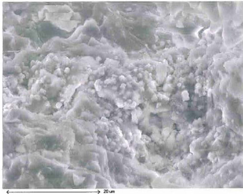
Figure 3 Iron-Rich Cubes (possibly ankerite) Shown at x2200 by Scanning Electron Microscopy (Actlabs, 2006)
