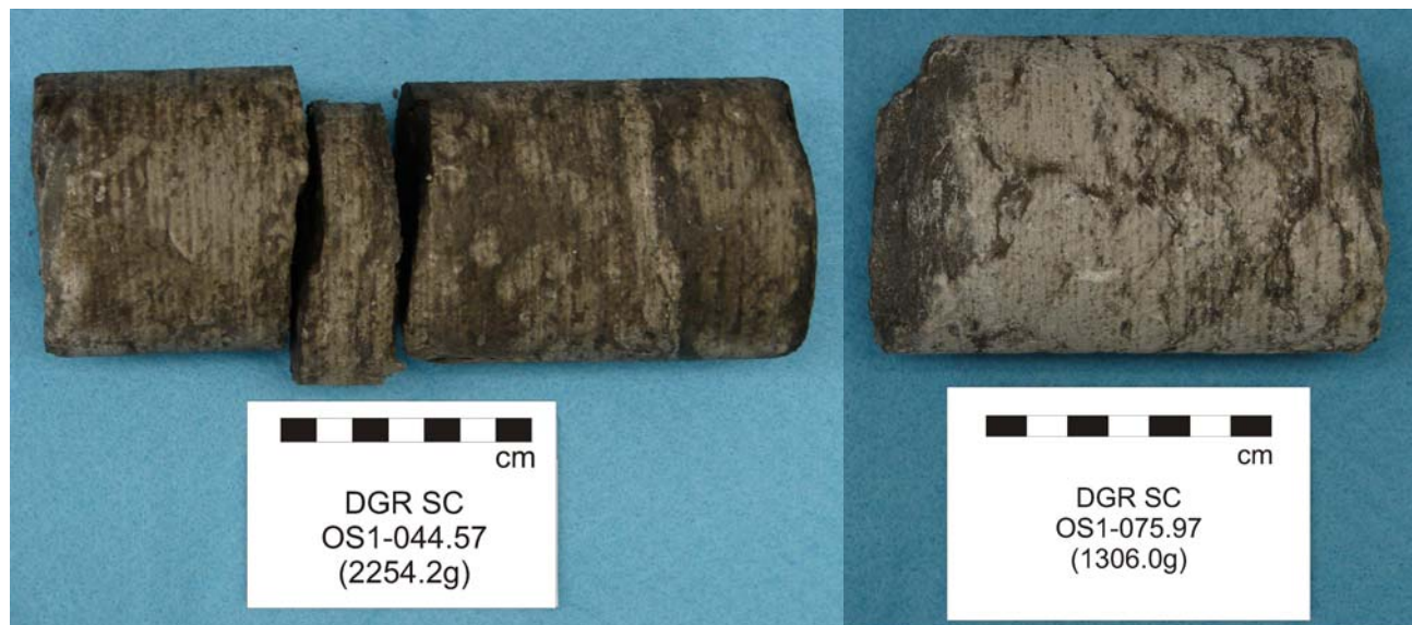
Figure 9 Saturated Core Samples from Borehole OS1, St. Mary's Cement Quarry, Bowmanville
